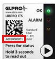
The Configuration Profile can be identified via the first four characters of the Device ID
