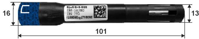
Dimensional view of the two variants: temperature / humidity sensor
