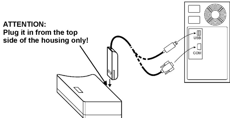
After connecting the datalogger to the computer, evaluation and programming of the datalogger is possible, by the elproLOG software.
