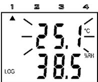
Active alarms are indicated (if the display is on), by blinking of the value on the display and an arrow symbol appears at the measuring channel.
