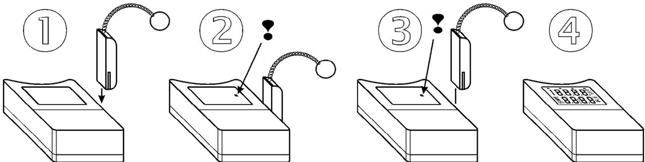
**If the datalogger is in the Start/Stopp mode and is waiting for the start, the display is blanc!**
