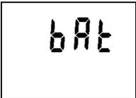
If BAT is displayed permanently, the battery voltage is too low and the datalogger may not be started. If the datalogger is running, the recording will stop. Communication with the computer may temporarily work. **Replace battery as soon as possible!**
