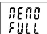
If the memory is full in the Start-Stop mode, the recording will be stopped and in the message MEMO FULL is displayed. This message is going to be displayed even the datlogger is in the power save mode.
