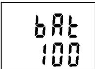
Afterwards the estimated, remaining battery capacity (values 0 to 100%) is displayed for approximately 2 seconds.
