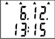
Warning: date / time display: after a battery voltage drop, e.g. battery exchange, all 4 arrows show up in the display. However all datalogger functions are working without any limitations. Check date and time and if necessary set them by the elproLOG software.
