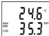
**If the display is switched on** actual measurement values of both sensors are displayed. The symbol LOG indicates that data logging is in progress – if it blinks, the data memory is filled up to more than 90%. The MIN / MAX values indicate the recorded extreme values.
