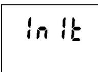
The indication INIT may appear after e.g. replacing a totally discharged battery. It will stay on for about 12 seconds (after the display test).
