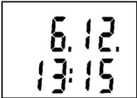
After the display test the actual date and time of the datalogger are displayed for approximately 4 seconds.
