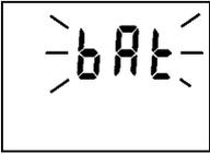
If a blinking BAT is displayed (for 1 second in a 10 seconds interval), the end of the estimated battery life is near. Replace the battery as soon as possible!
