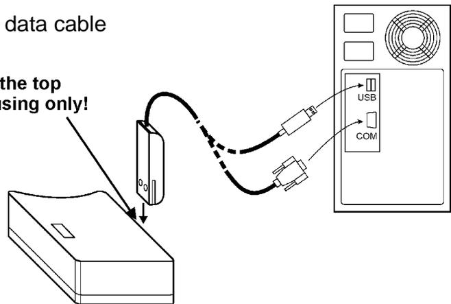
After connecting the datalogger to the computer, evaluation and programming of the datalogger is possible, by the elproLOG software.
