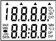
After reprogramming the datalogger, all LCD segments are switched on as a display test.
