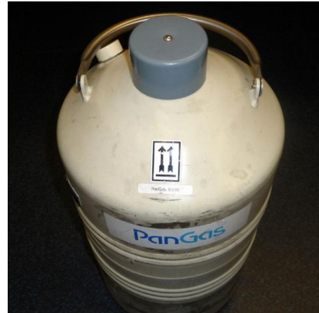
Liquid Nitrogen in LN2 tank.
