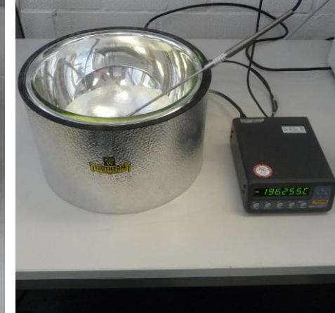
Check LN2 temperature with the reference instrument. Depending on the atmospheric pressure, it will show a temperature between -195^{\circ}\text{C} and -197^{\circ}\text{C} . Cover the top with a styrofoam to prevent from strong boiling.
