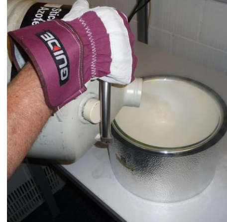
Fill dewar flask with LN2, about 10 cm deep. Take care – wear gloves.
