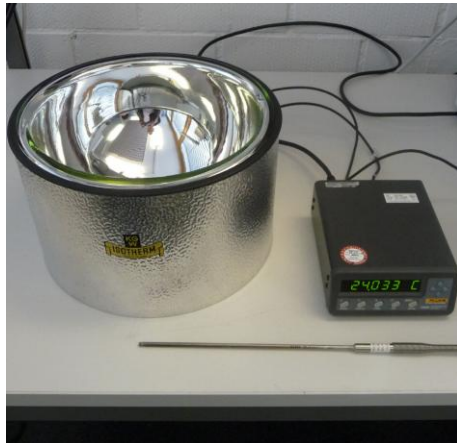
Dish-shaped dewar flask with certified reference instrument.
